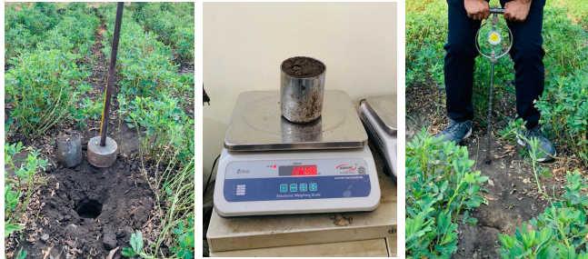
(a). Bulk density using core cutter (b). Weight of soil (c). Cone penetrometer
